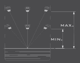
The nozzles are spaced using predesigned piping depending on the discharge flow rate. Each type of hazard has a specific nozzle with a given flow and coverage. For example, there are specific nozzles for fryers, ducts, filters, grills, burners, etc.
